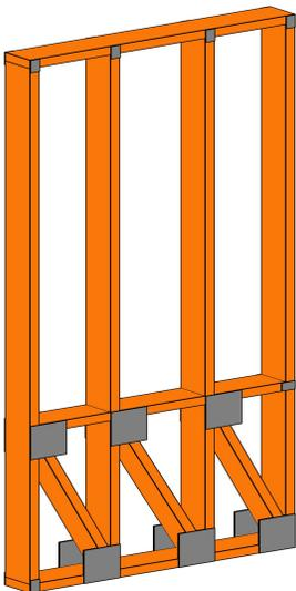
PSP™ Parapet Shear Panel
